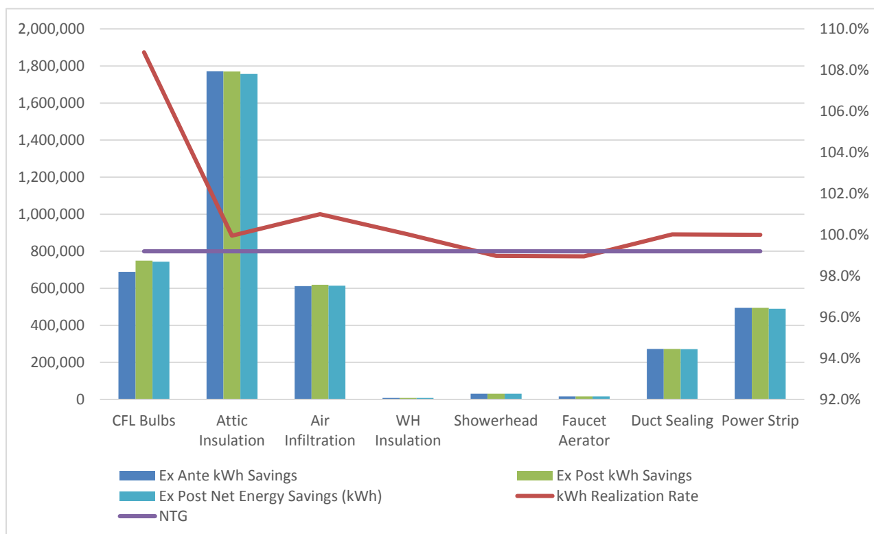
Figure 4-9 Unified Wx Energy Savings (kWh) Summary
